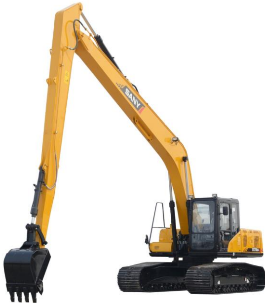
Long reach excavator
