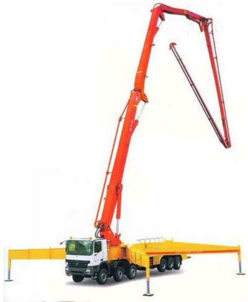
Boom concrete pump
